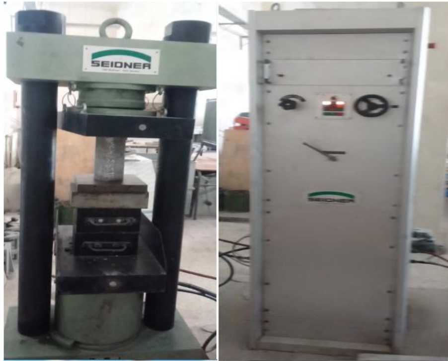
Figure III.3 : Essai de compression uni axial
