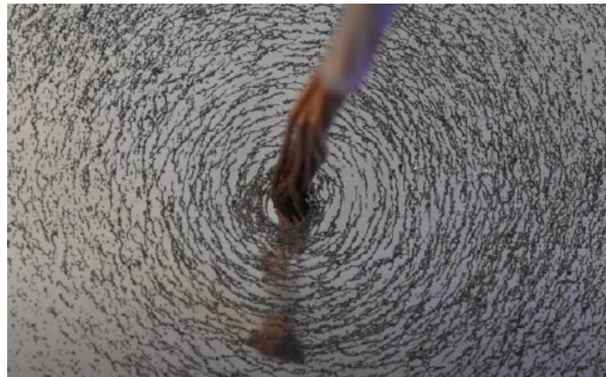
Figure 7.1: Imprinting the magnetic field of a current-carrying wire using iron filings (credit).
