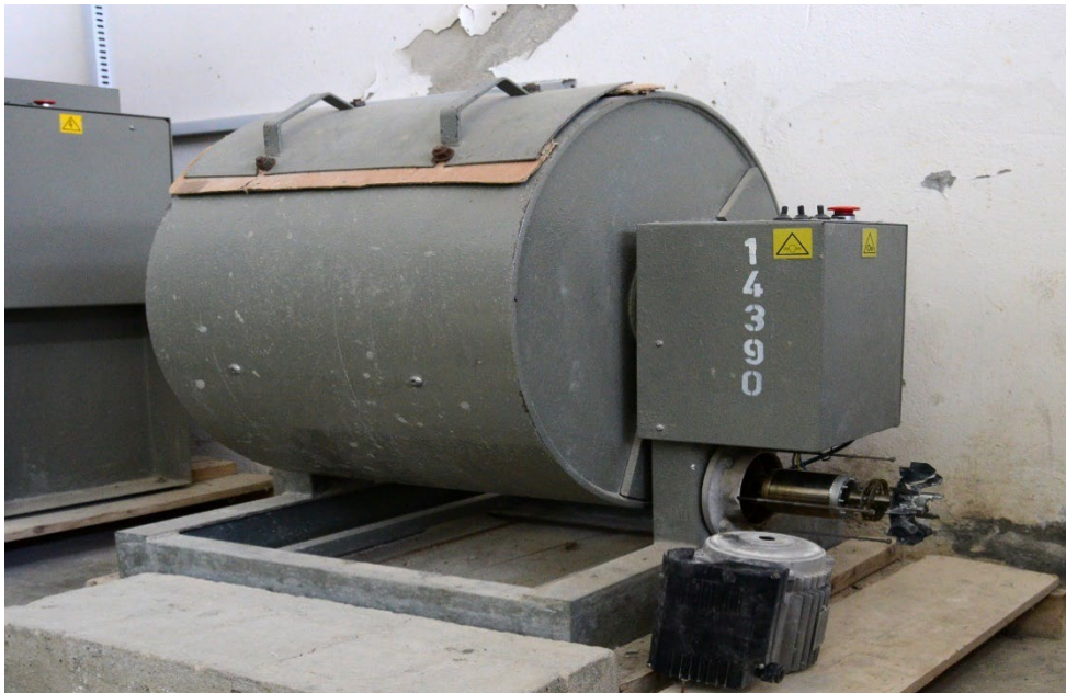
Figure III.9: Essai Los Angeles
