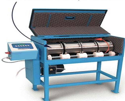
Figure III.11: Essai Micro Deval
