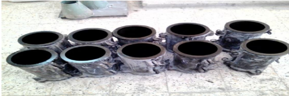
Figure II-11: Moules cylindriques (15x30) cm 2 .
