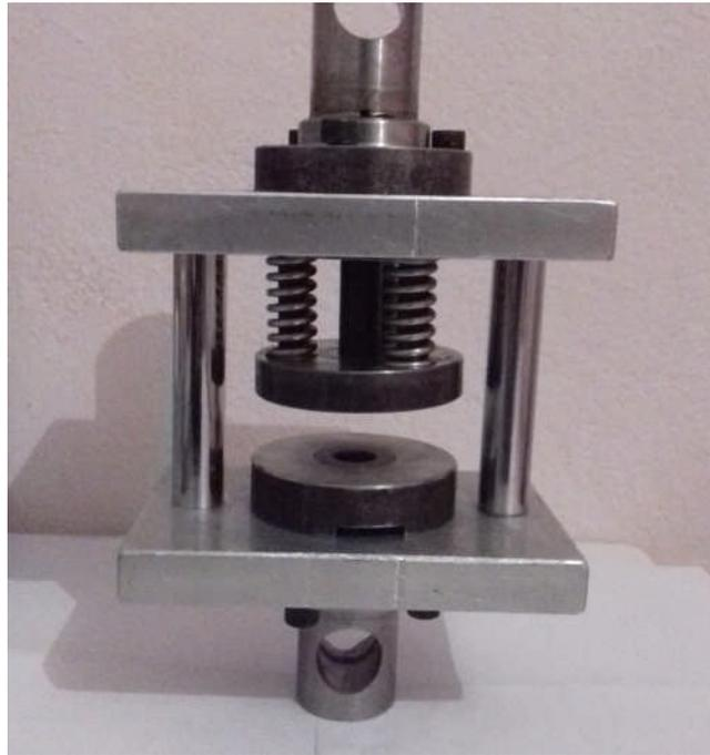
**Fig.IV.7 :** Assemblage poinçon/matrice
