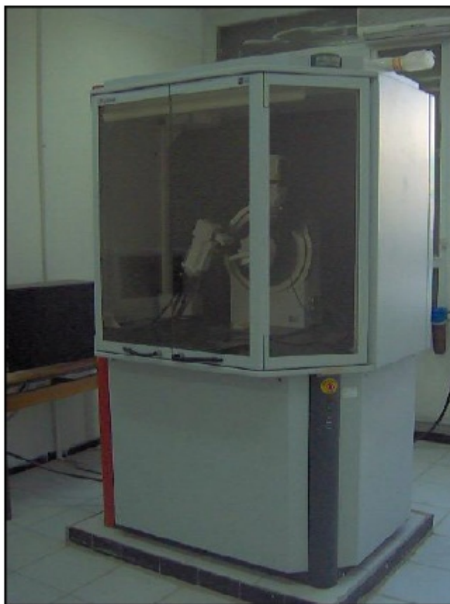
Figure. III.14 : Photographie du diffractomètre Bruker AXS D8 Advance.
