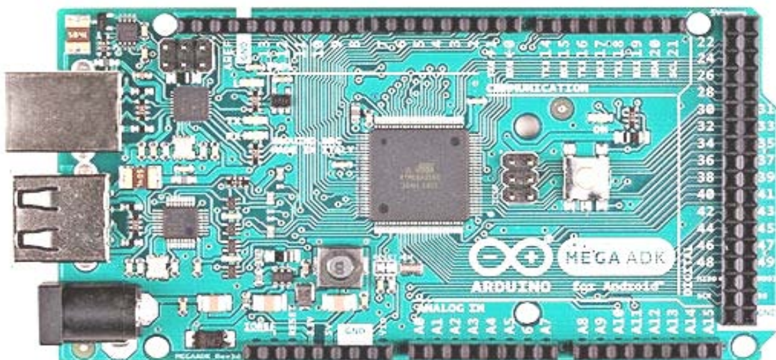
Figure II.1: Carte Arduino Méga (ADK) [8]
