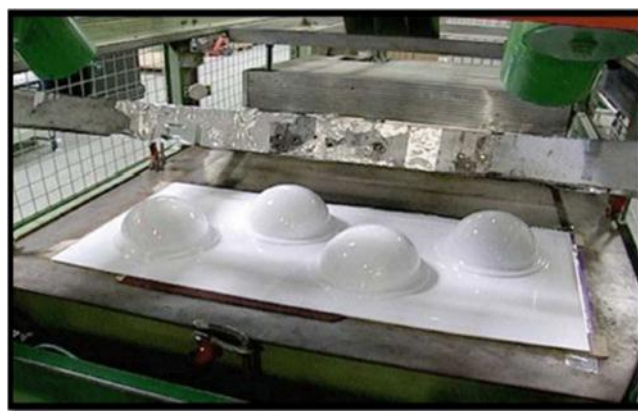
Figure I.15 Cycle de thermoformage
