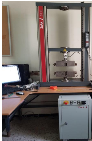
Figure III-7 : Machine de traction ZWICK/Z010.
