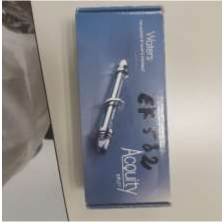
Figure 25 : colonne griffée ACQUITY UPLC BEH C8, 2.1 * 100 mm
