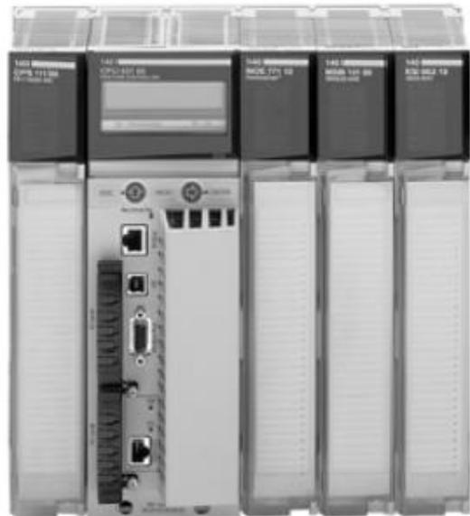
**Fig. A.7 : Automate Modicon Quantum**
