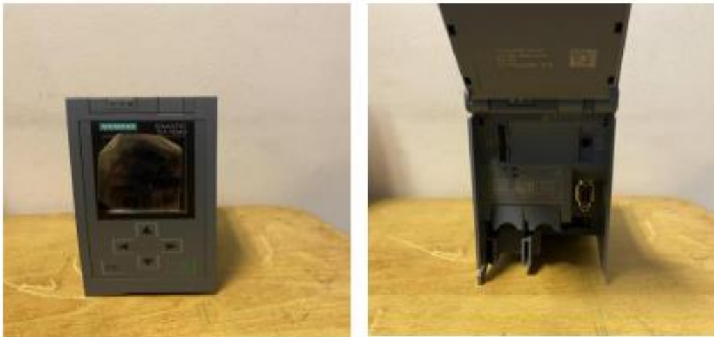
Figure III- 10 : Automate programmable industriel (API)
