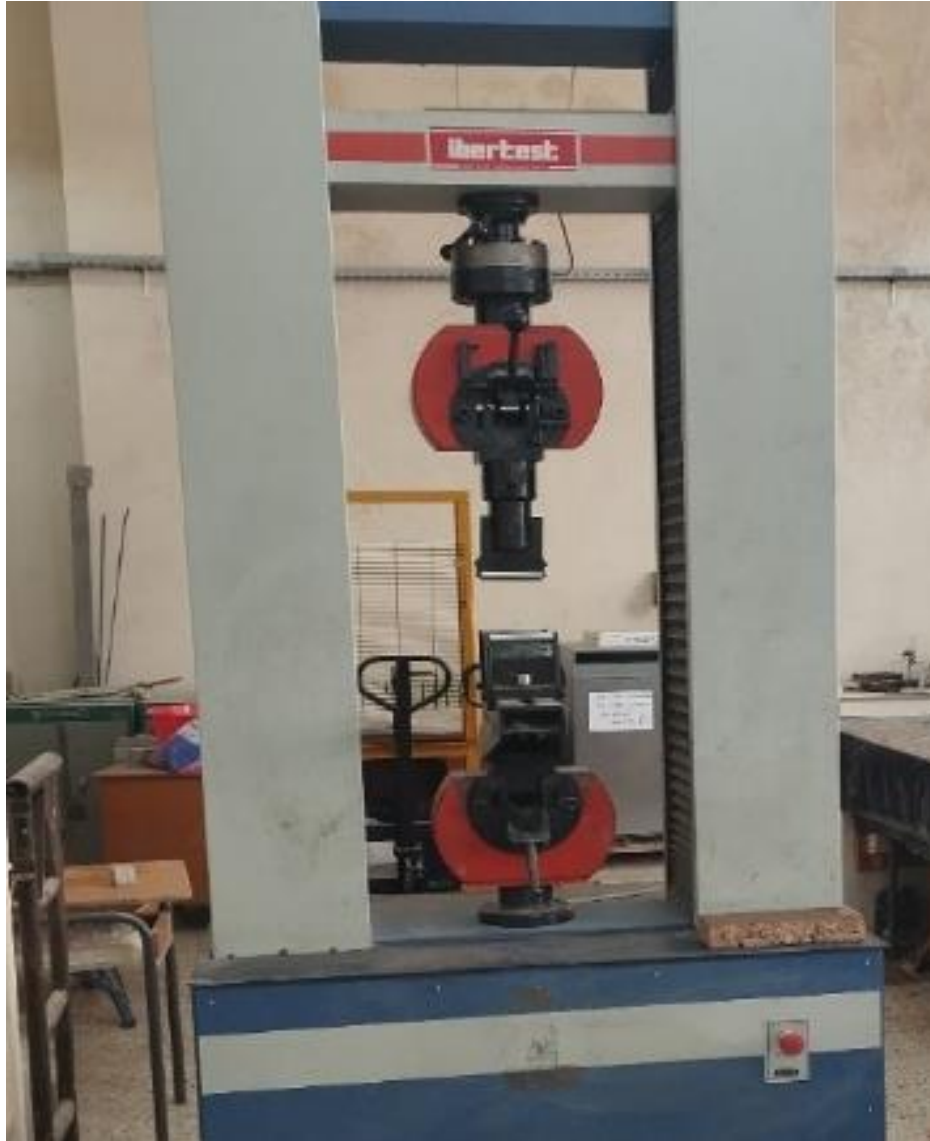
Figure II-14: machine de flexion type IBERTEST MOD
