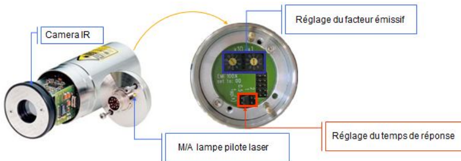
Figure II.13.a : composant de la camera
