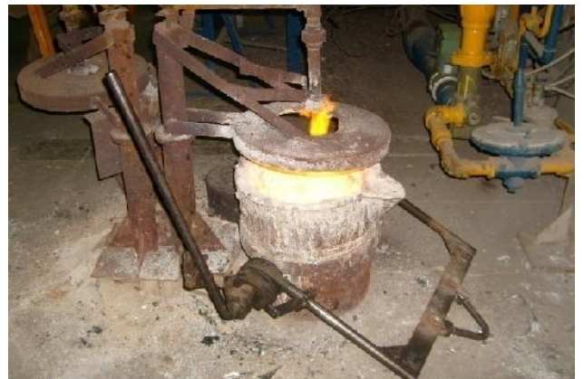
Figure II.1.5. Poche de coulée
