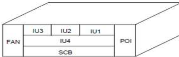
OptiX 155/622H slot layout
