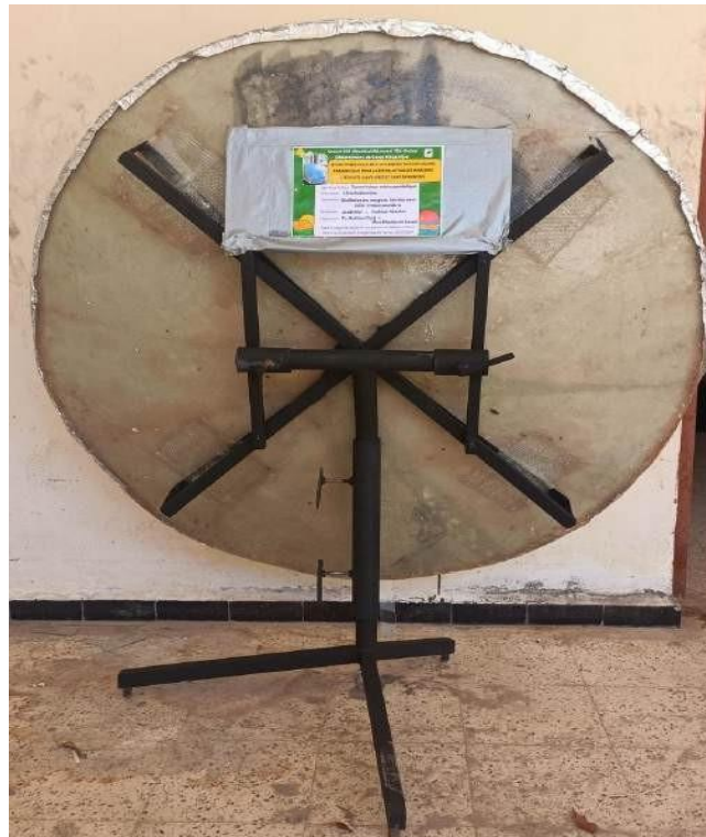
Figure IV-32 : Support de la parabole
