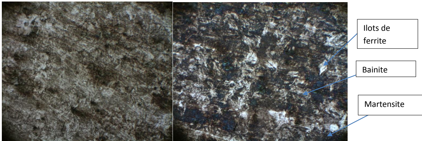
Figure IV.21. Microstructure de la ZAT G.x 100
