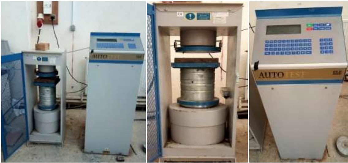
**Figure IV.29.Machine de compression Autotest.**
