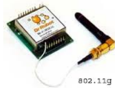
Figure II.15 : Module WFS802G série (802.11g)
