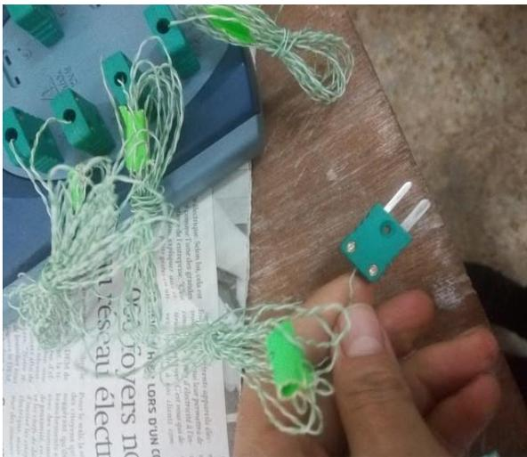
Figure III-19 : Thermocouple type K
