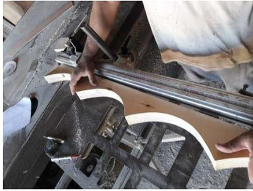
*Figure IV.13: support cylindro-parabolique.*
