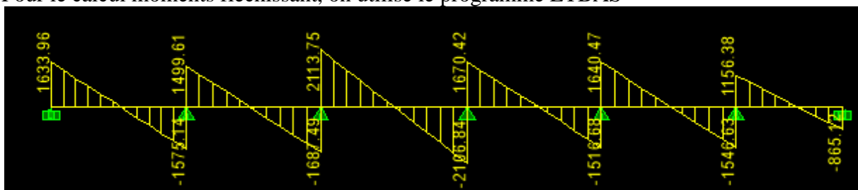
Figure IX.6. Diagramme des efforts tranchants ELU :
