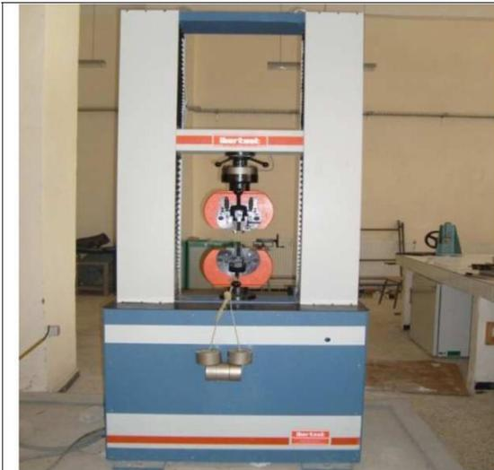
Figure II.1.20 - Machine de traction
