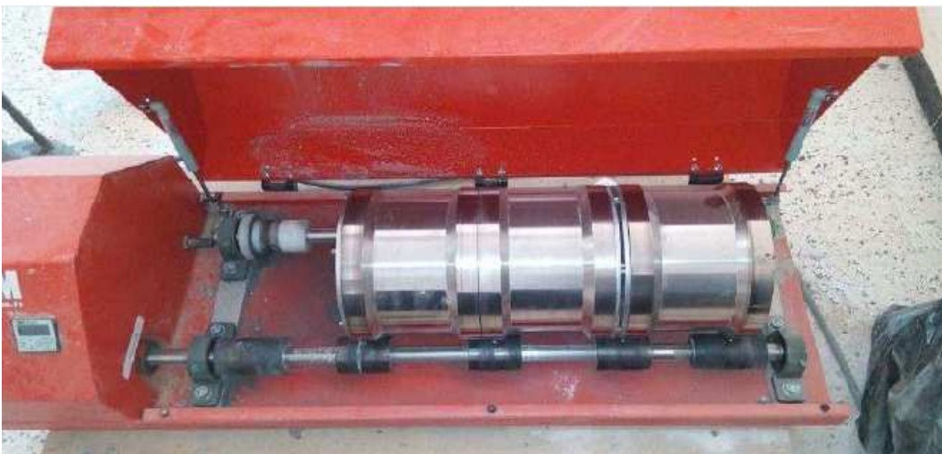
Figure 1.V. Appareillage Micro Deval.
