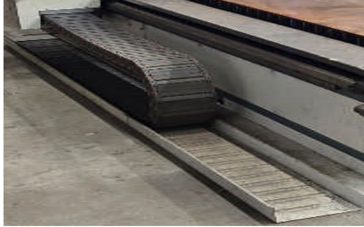
Figure □ - 24: chaine porte câbles
