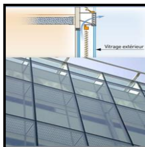
Fig.180. Façade double peau Source : https://www.google.com/search?q=facade+doublepeau
