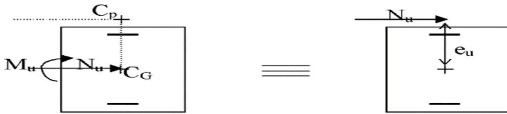
Figure III.2.4: position du centre de pression
