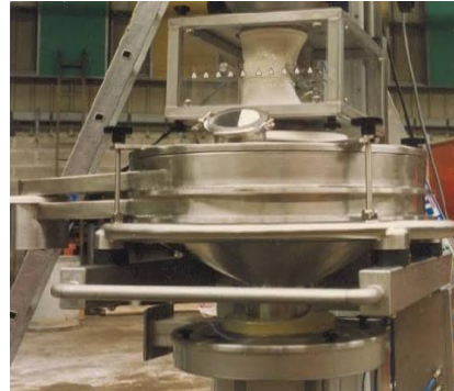
Figure 2 : Tamis vibrant CMA
