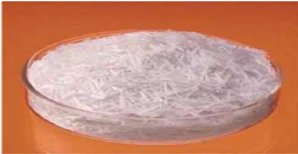
Figure I.14: Fibre de verre [12].
