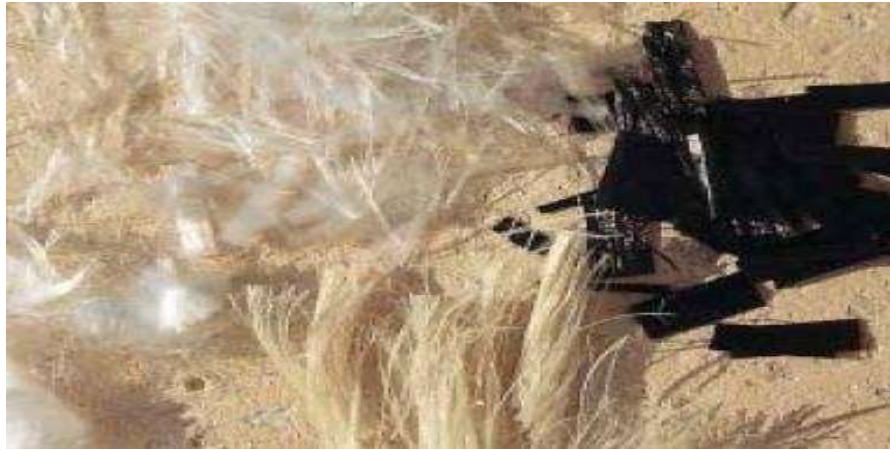
Figure I.13: Fibres de polypropylène [14]
