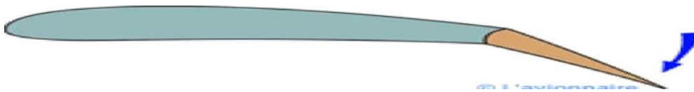
Figure III. 31 Volet de courbure. [48]
