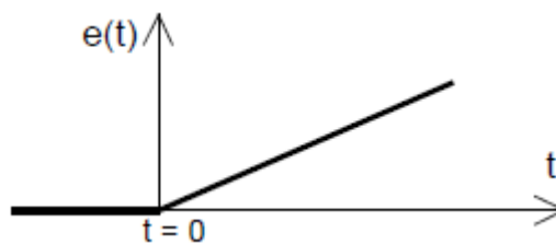
Figure 1-5. Signal en rampe
