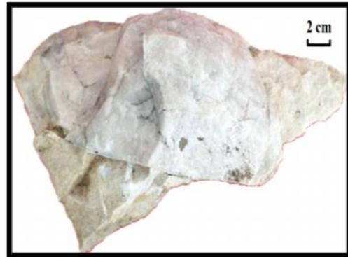
Figure V-4: Echantillon de barytine massive.
