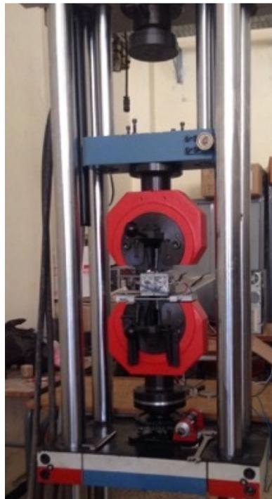
Figure 2.6 – Machine hydraulique IBERTEST.
