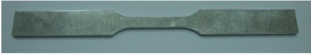
Figure 1.9 – Eprouvette de traction plane.
