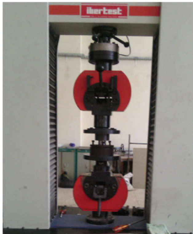
Figure III.3 : machine de traction –compression
