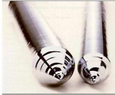
Figure 1.5: lingots de Si monocristallin [10].
