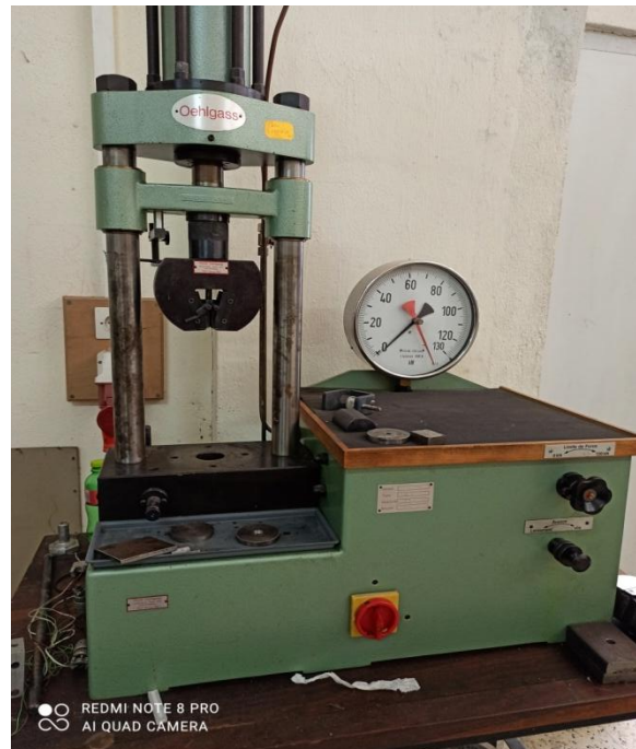
Figure III.4 : machine de traction hydraulique
