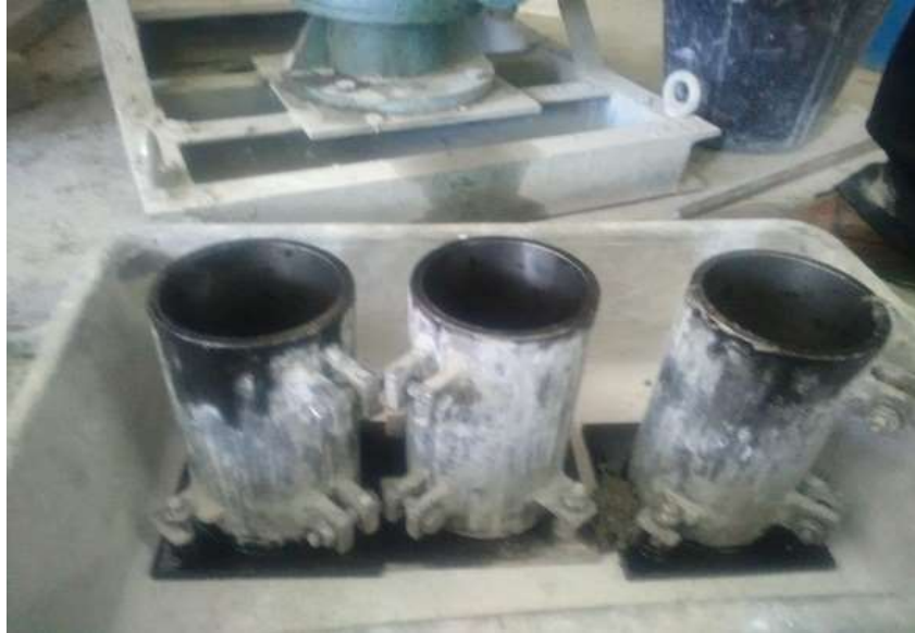
Figure II.5 Moules cylindriques (10×40) cm
