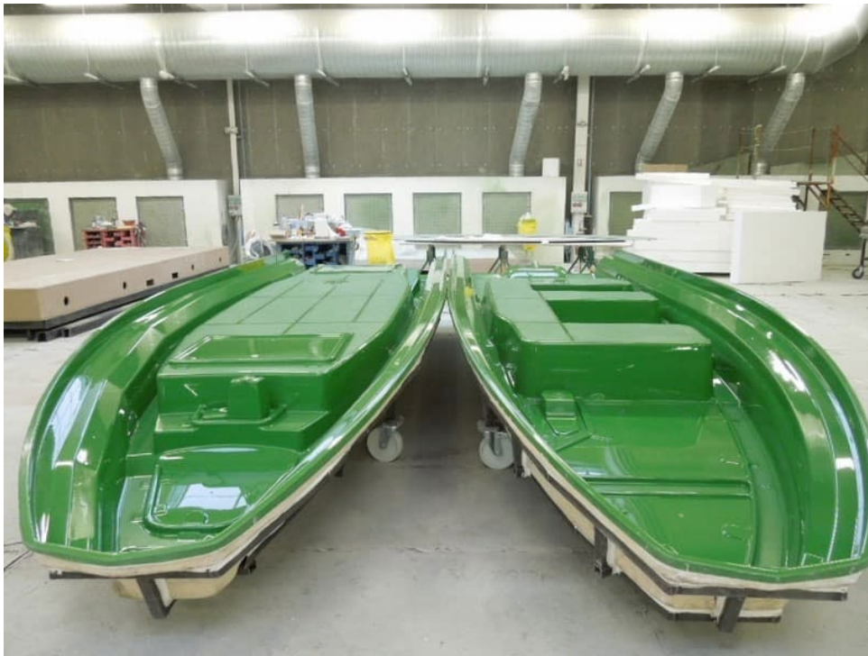
Figure 24: moule coque de bateau
