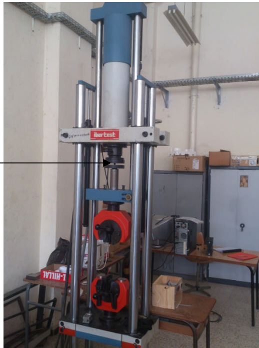
Figure 4.21 : Machine de traction/compression de type Ibertest.
