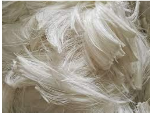
Figure I-9 fibre de verre
