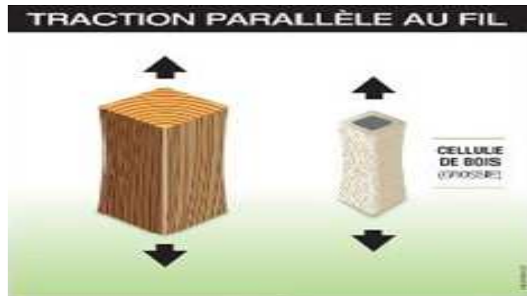
Figure 1 .13 : Contrainte de rupture de traction axiale.
