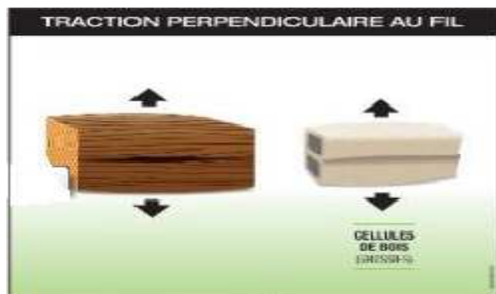
Figure 1.14 : Contrainte de rupture de traction transversale.
