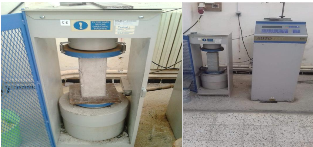
Figure. II.17: Eprouvettes soumise la compression.
