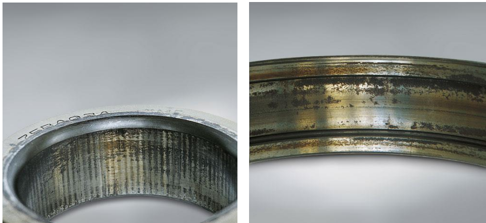
Figure II.15 : corrosion des pistes. [7]
