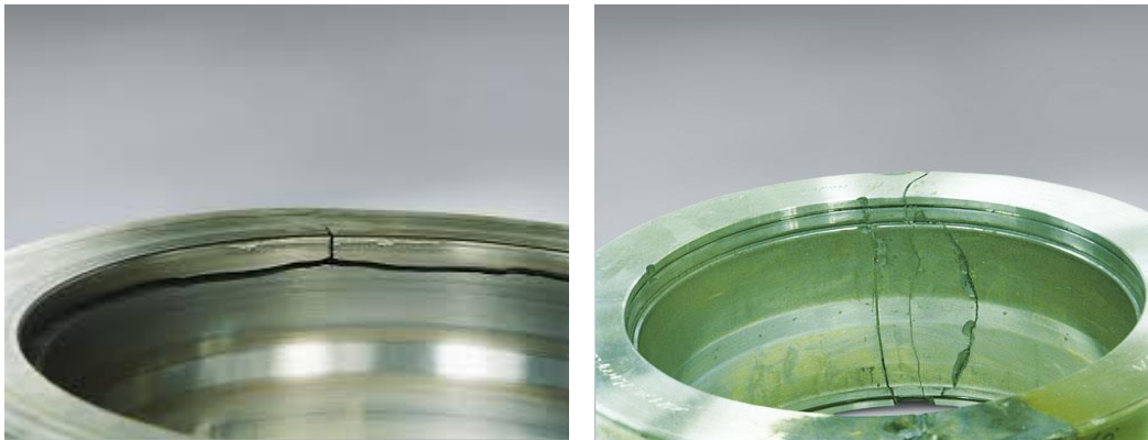
Figure II.11: fissure et cassure des bagues. [7]
