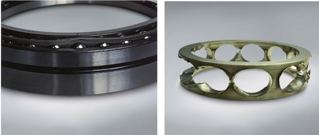
Figure II.12: détérioration de cage. [7]
