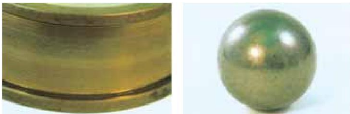
Figure II.21: taches et décoloration. [7]
