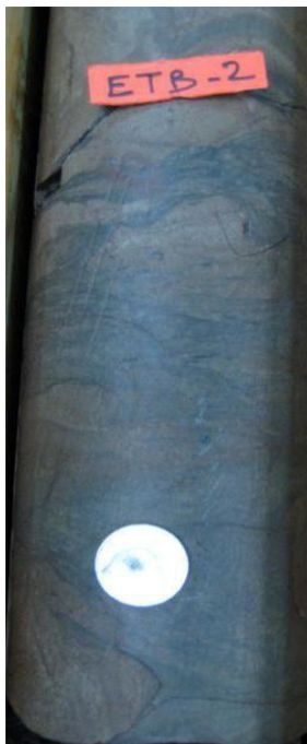
Figure.19 : Les convolutes (Slumps) ETB-2, C2, 3438-3439 m
