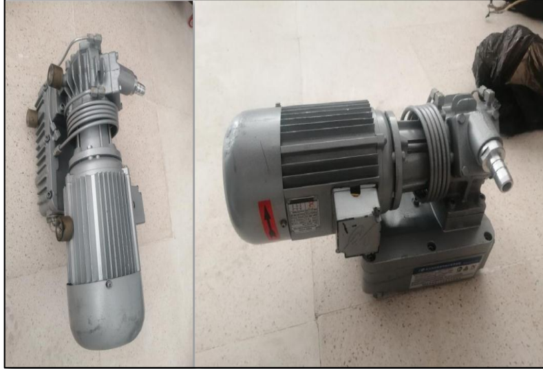
Figure III.26: Pompe à vide
