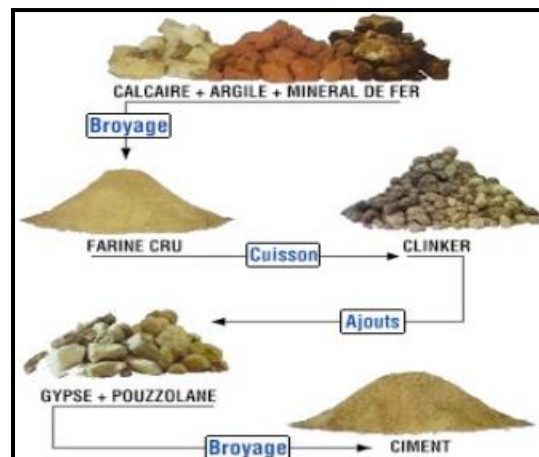
Figure II.13. Processus de fabrication de ciment
