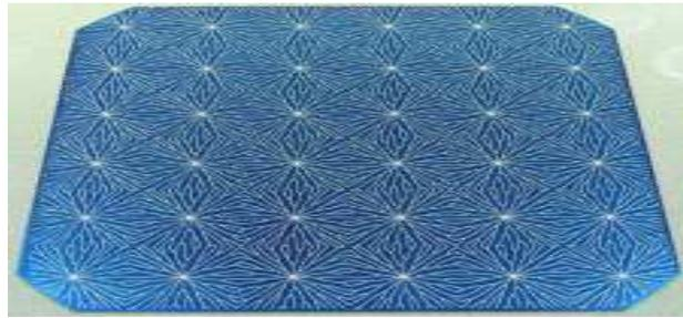
Figure I-10. Cellule MWT
