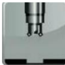
Figure I.10 : Surfaçage et rainurage
