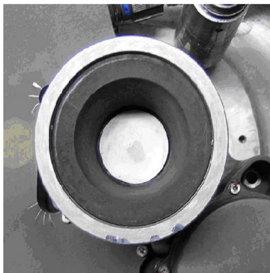
Figure 2-3a opercule de tuyère - AASM
